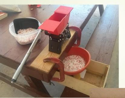
**Step 1**: Collect left over and disused filament (white bowl, left). Put them into the top of the grinder (red box, center) and crank the silver handle until ground plastic pellets are fall into (red) bowl.
